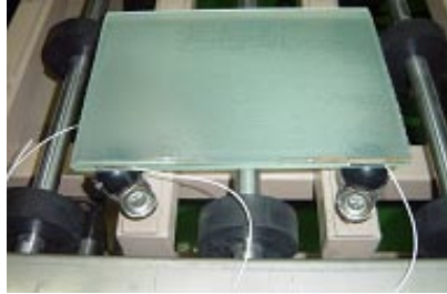
[Wiring work after autoclave]
